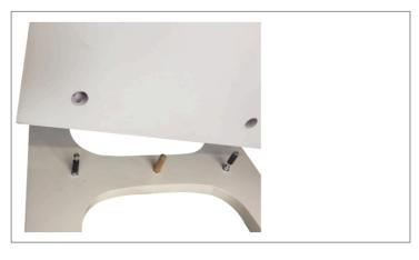
Now insert the slabs into the sides (bolt holes facing downwards)
